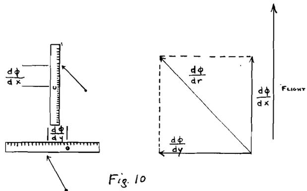
passed through the center of the thermal. Now to obtain maximum lift after passing through the center he turns until his lateral gradient becomes a maximum and his longitudinal zero. He is thus following one of the isotherms.
